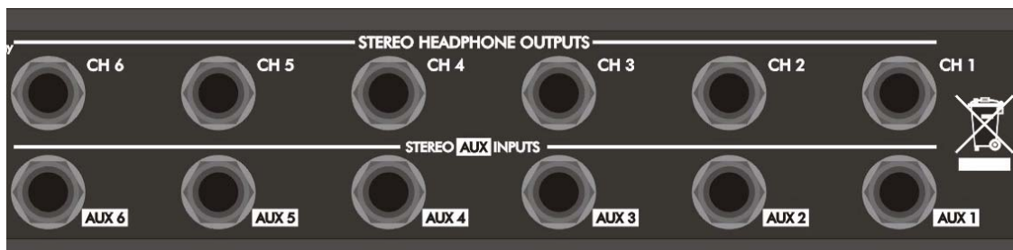
FIGURE 3 - Rear Panel Headphone Outputs and Aux Inputs
