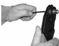
Installation of BNC Connectors LA-114
